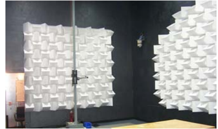
Hybrid on Ferrite Absorber in FCC Filed 3 Meter EMC Chamber
