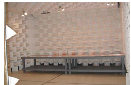
Hybrid on Ferrite Absorber in a Multi-Purpose EMC CISPR25 / MIL461 / Avionics Test Chamber
